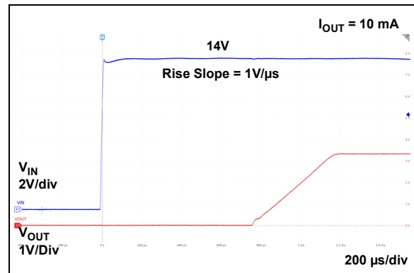
FIGURE 2-28: Start-up From V_{IN} (0V to 14V, V_R = 3.3\text{V} ).
