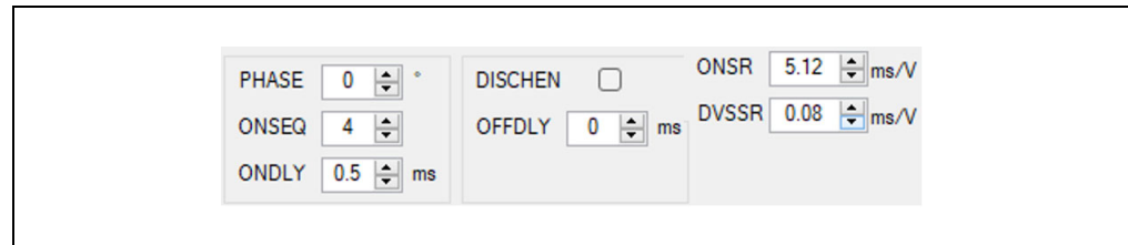
FIGURE 4-14: Start-up, Shutdown and Dynamic Voltage Scaling Settings for Buck Channels.
