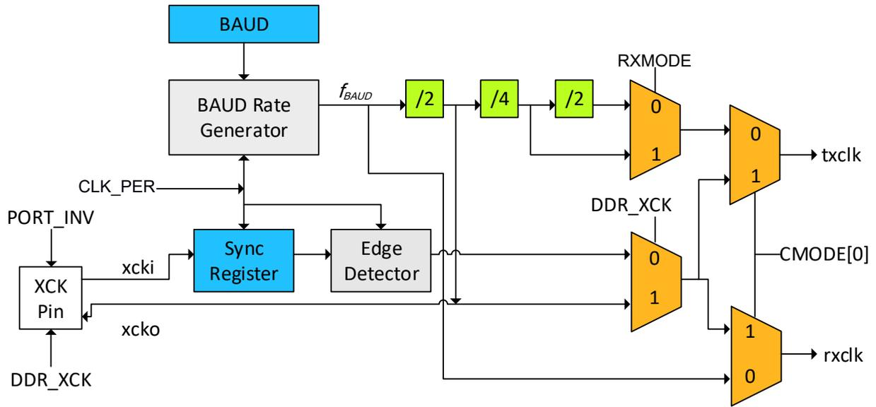
**Internal Clock Generation - The Fractional Baud Rate Generator**
