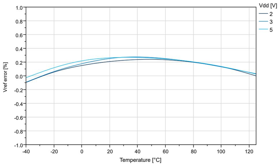
**Figure 32-33. Internal 2.5V Reference vs. Temperature**
