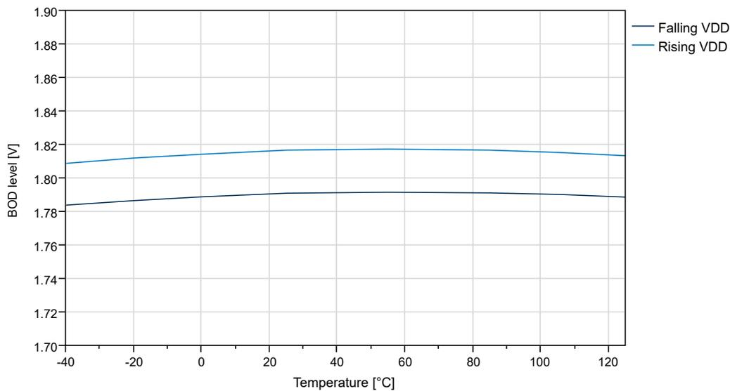
Figure 32-39. BOD Threshold vs. Temperature (Level 2.6V)
