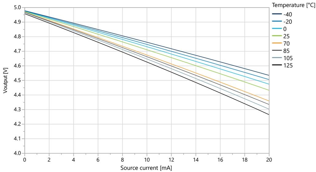
**Figure 32-27. I/O Pin Output Voltage vs. Source Current (T=25°C)**
