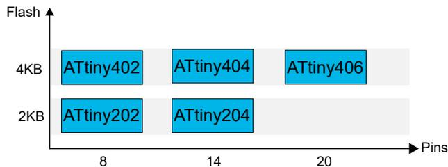
The fully compatible variants of the ATtiny devices, that is the vertical migration option shown in the figure above, come with both smaller and larger Flash memories.
