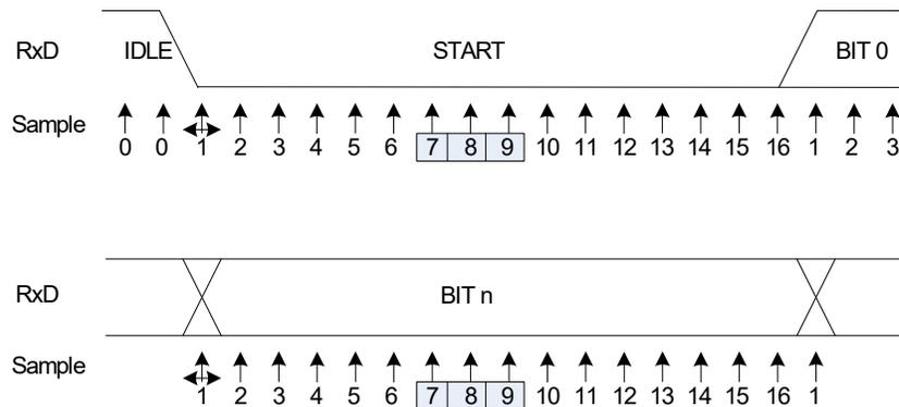
The transmission baud rate must be set up in relation to the selected UPDI clock, which can be adjusted by UPDICKSEL in UPDI.ASI\_CTRLA. See [Table 30-2](#) for recommended maximum and minimum baud rate settings.
