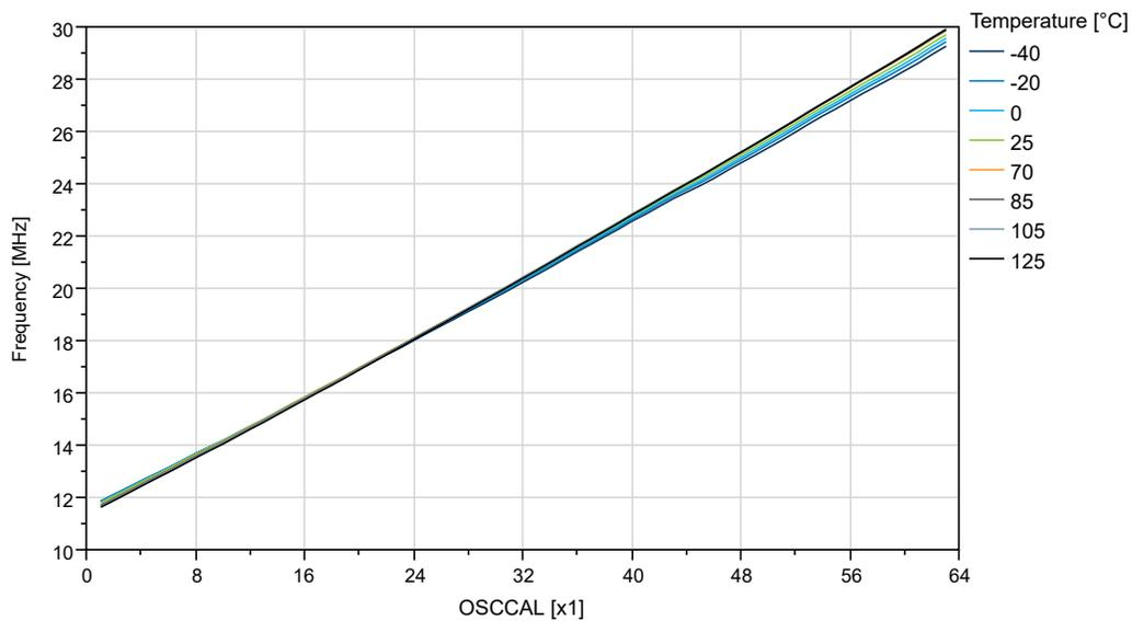
**Figure 32-59. OSC20M Internal Oscillator: Frequency vs. Temperature**
