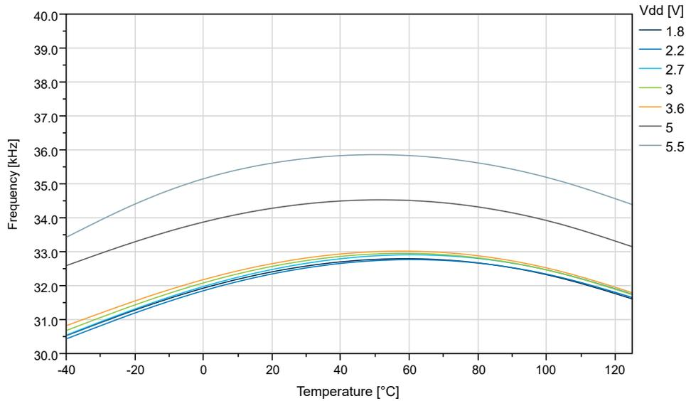
**Figure 32-62. OSCULP32K Internal Oscillator Frequency vs. V<sub>DD</sub>**
