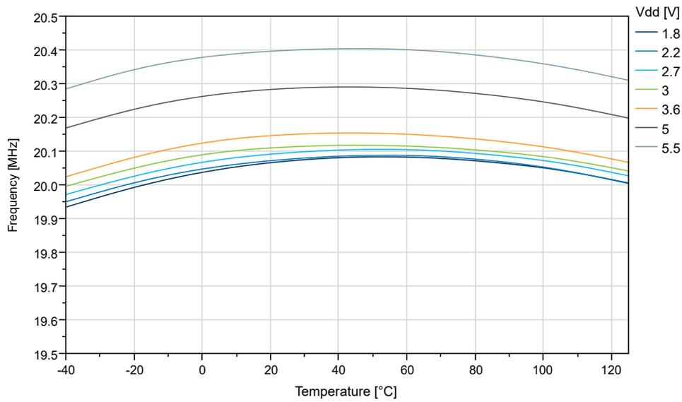
**Figure 32-60. OSC20M Internal Oscillator: Frequency vs. V<sub>DD</sub>**
