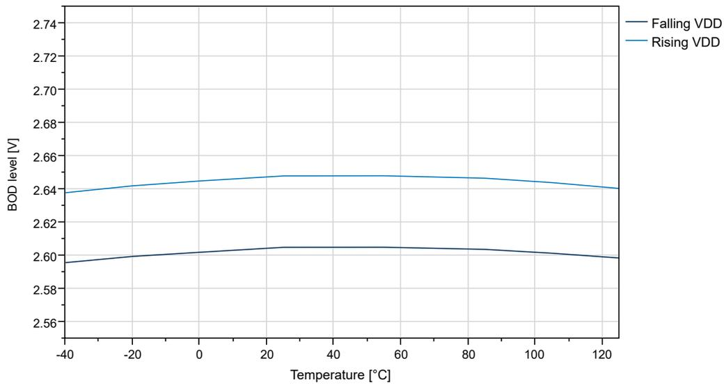
Figure 32-40. BOD Threshold vs. Temperature (Level 4.3V)
