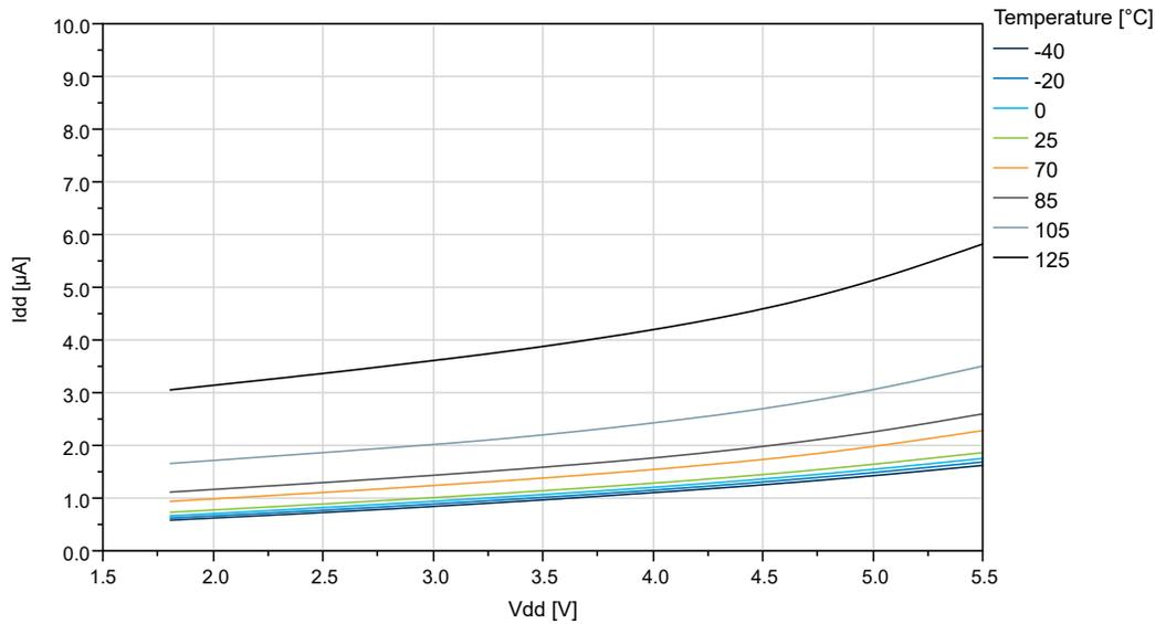
**Figure 32-13. ATtiny204/ATtiny404: Standby Mode Supply Current vs.  $V_{DD}$  (RTC Running with Internal OSCULP32K)**
