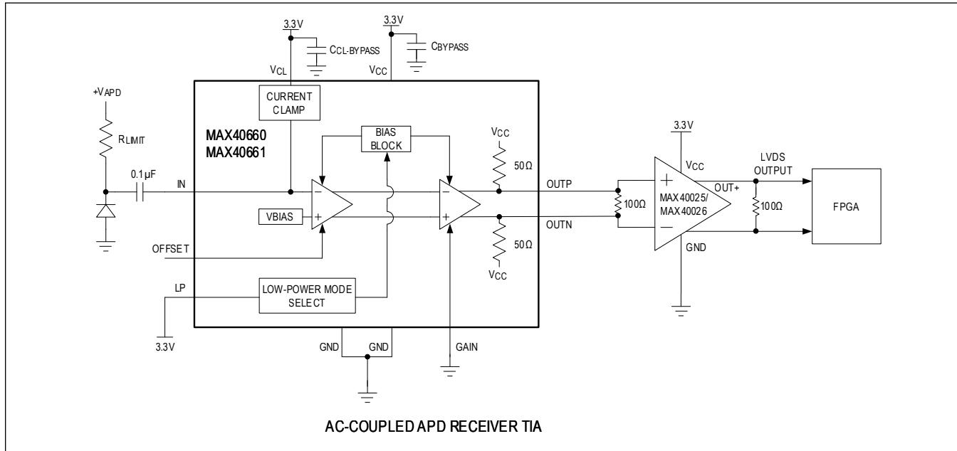
The APD's cathode is connected through a coupling capacitor to the TIA's input, with the anode connected to ground. The bias voltage in this case is positive, and is connected to the cathode through a resistor. Incident light pulses cause current to flow from the IN pin and into the APD. This input current also flows through an internal resistor to create a voltage, which is then amplified by the second stage to create a differential output signal that can drive a high-speed ADC or comparator.
