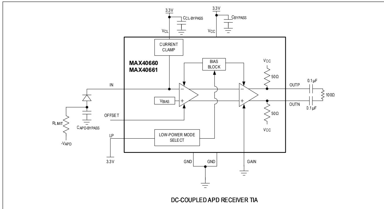
The APD's cathode is connected to the TIA's input, and the anode is connected to the negative bias voltage through a resistor. Incident light pulses cause current to flow from the IN pin and into the APD. This input current also flows through an internal resistor to create a voltage, which is then amplified by the second stage to create a differential output signal that can drive a high-speed ADC or comparator.
