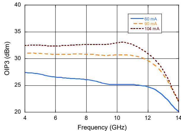
Typical Performance Curves:  $V_{CC} = 5$  V,  $+25^\circ\text{C}$
