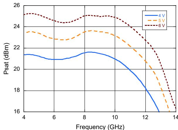
Typical Performance Curves:  $I_{CC} = 90$  mA,  $+25^\circ\text{C}$
