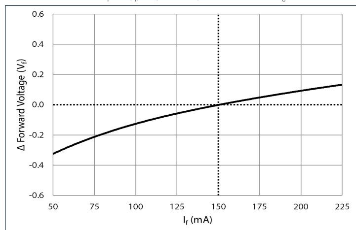
Temperature:  $\Delta V_f = V(T_c) - V(25^\circ\text{C})$ , 20 ms pulse,  $I_f = 150 \text{ mA}$
