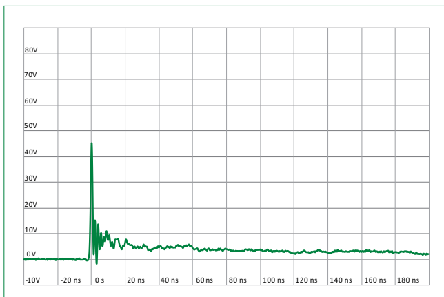
ISO10605 Contact Discharge Plot at +8KV
