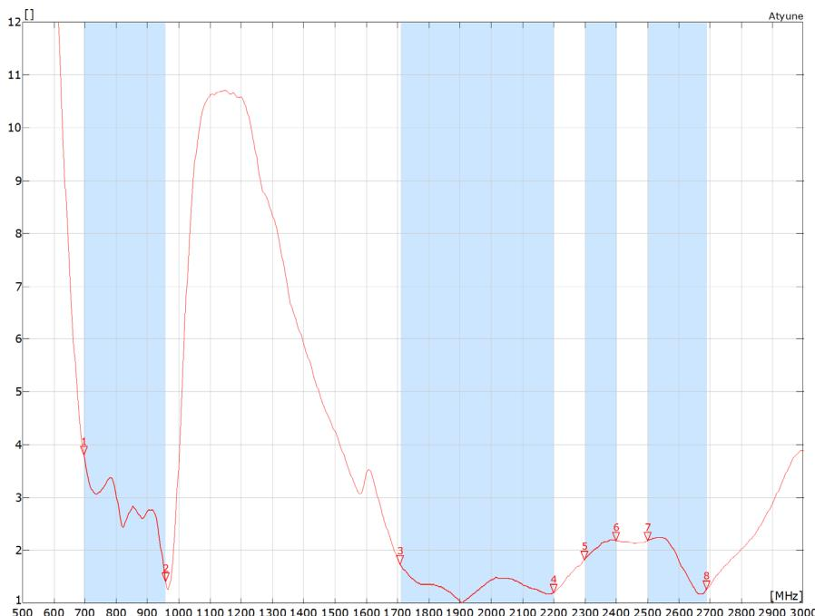
All data measured on Antenova's evaluation PCB Part No. SR4L073-EVB-1 (EVK size 60mm x 40mm)
