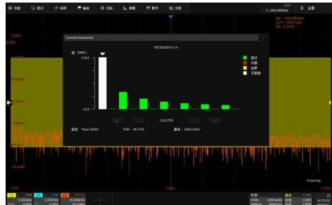
The Power Analysis application provides a full suite of power measurement and analysis tools. These tools enable an improvement in the efficiency of measurements made on switching power supplies and power devices. The Power Analysis application can measure Power Quality, Current Harmonics, Inrush Current, Switching Loss, Slew Rate, Modulation, Output Ripple, Turn On/Off, Transient Response, PSRR and Efficiency. Each measurement has a help screen showing a connection diagram with notes.
