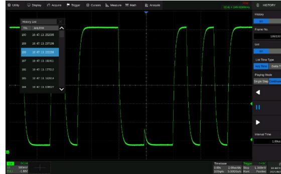
The history function can record up to 80,000 frames of waveforms. The recording is executed automatically so that the customer can playback the history waveforms at any time to observe unusual events and quickly locate the area of interest using cursors or measurements. The failed frames of the Mask Test can be stored as history frames.
