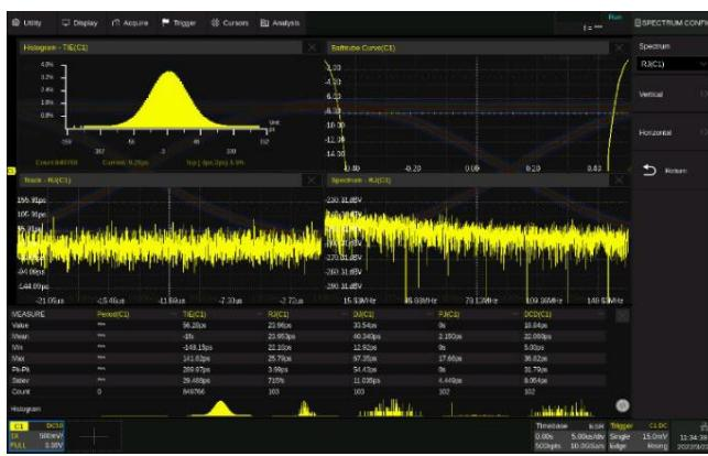
Supports eye diagram and jitter analysis/measurement. It can automatically extract the embedded reference clock from serial data and create an eye diagram. Measurement on multiple eye/jitter parameters is provided and mask testing of eye diagrams is supported.
