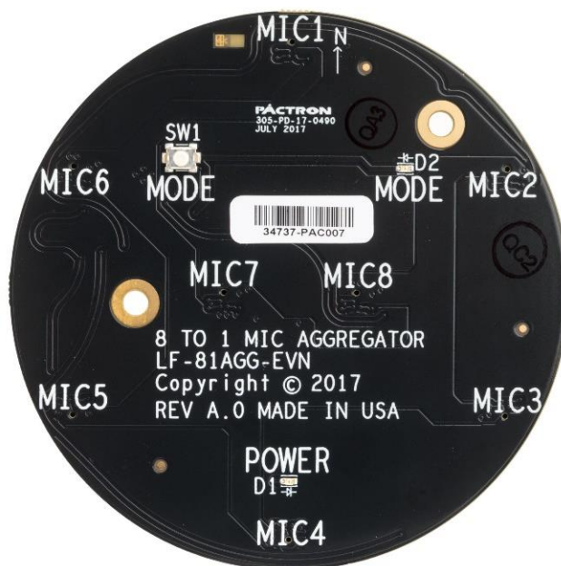
Figure 6.2. 8 to 1 Mic Aggregator Board (Daughter Board)
