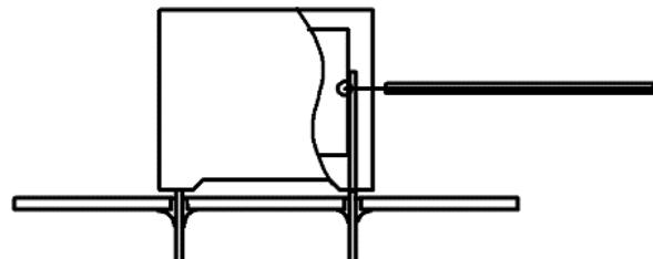
Temperature monitored inside the capacitor.
