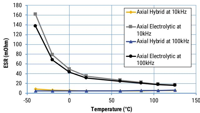
Temperature dependencies of ESR measured at 10 kHz and 100 kHz for Axial Hybrid (PHA225MKP3370QE4) and Axial Electrolytic (PEG226MG3370QE1) capacitors.
