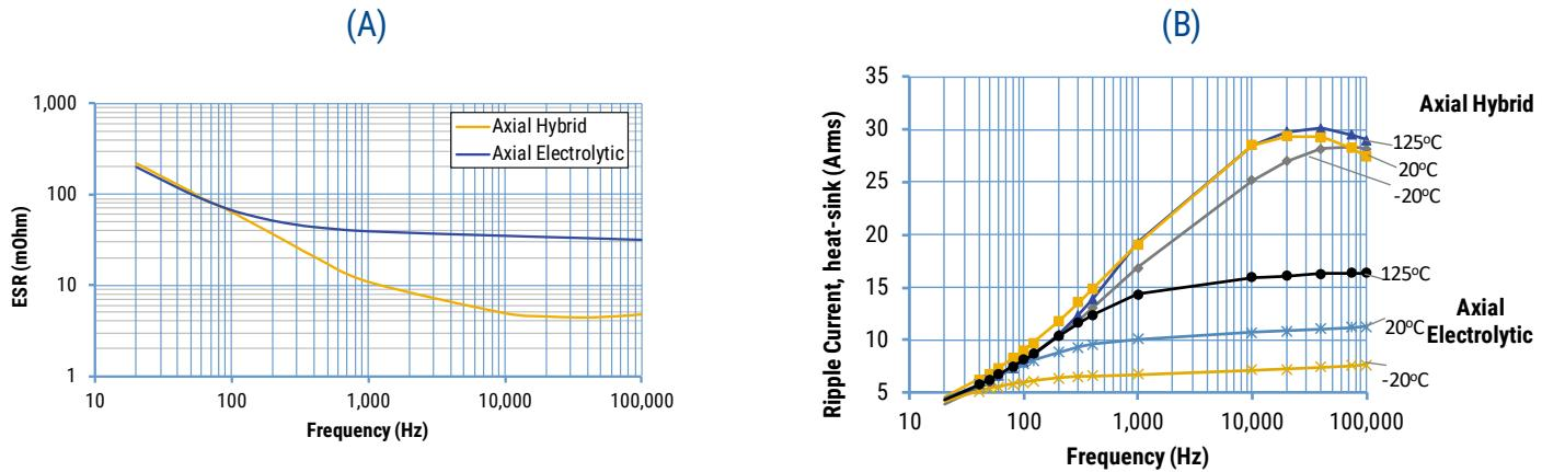
Frequency dependencies of ESR measured at 20°C and 100 kHz for Axial Hybrid (PHA225MKP3370QE4) and Axial Electrolytic (PEG226MG3370QE1) capacitors (A); Frequency dependencies of max. short pulse Ripple Current at different temperatures for heat-sink mounted Axial Hybrid (PHA225MKP3370QE4) and Axial Electrolytic (PEG226MG3370QE1) capacitors (B).
