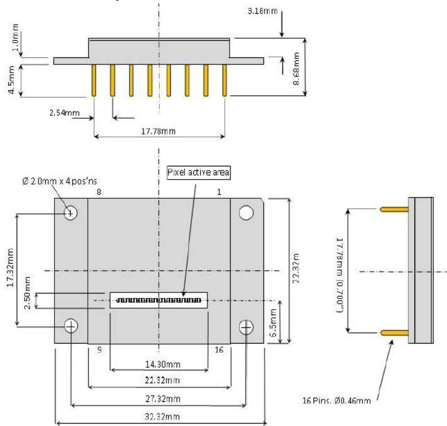
**Pin Configuration of Sensor - 255 and 128 Element Line Sensor Array**
