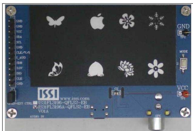
Figure 1: Photo of IS31FL3196A Evaluation Board
