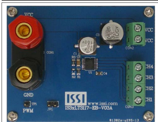
Figure 1: Photo of IS31LT3117 Evaluation Board
