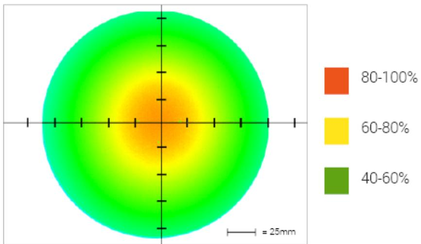
Optical measurement taken using RL208M-100WHIIC @ 300mm
