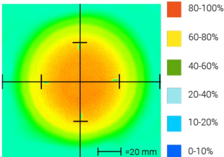
Optical measurement taken using DF196-100WHII3 @ 25mm
