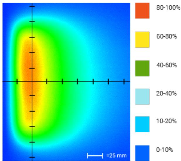
Optical measurement taken using AL4554-660C5 @ 25mm
