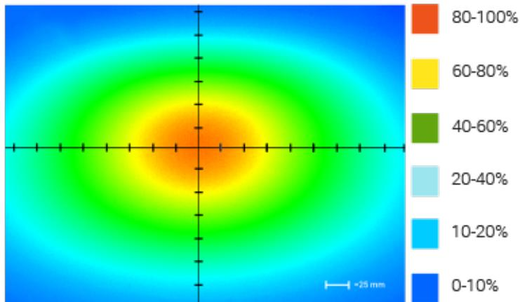
Optical measurement taken using AL126-WHIIC Rev. A @ 200 mm
