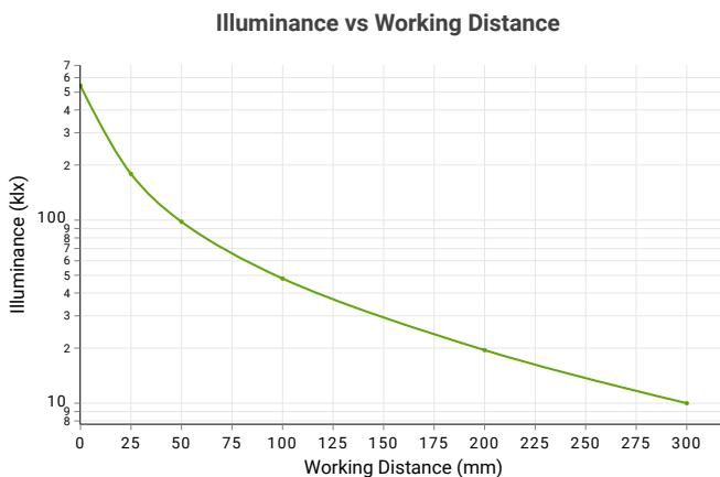
Linear Backlights, while typically oriented behind the object of interest, can also be used for highly diffuse front illumination at short to medium working distances. The chart to the left shows the BL138's intensity as its distance from the inspection surface changes.
