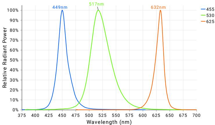
Visible color illumination consists of using wavelengths between 400-700 nm to either create or eliminate contrast on an inspection subject based on differences in a features color hue. When referring to a color wheel, simply remember the following; like colors reflect and brighten surfaces; conversely, opposing colors absorb and darken surfaces. The BL138 is available in **455nm, 530nm, and 625nm** visible color configurations.
