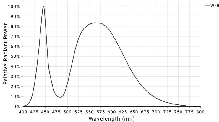
White LED illumination is the most commonly used machine vision lighting configuration. It is often the default choice when specific features of interest do not require color-based highlighting. However, **white LEDs can vary in color temperature between different lighting families, which can impact machine vision systems**, specifically when matching white light sources.
