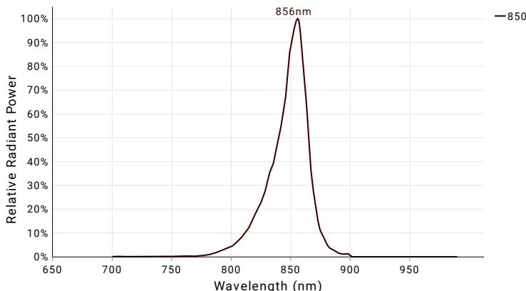
Near-infrared (NIR) imaging is a machine vision technique using longer wavelengths of 700-1000 nm to penetrate specific materials that are otherwise opaque to under the visible spectrum. When paired with a NIR camera, a NIR light can be ideal for applications such as fill level inspection, circuit board inspection, food safety inspection, and medical imaging.
