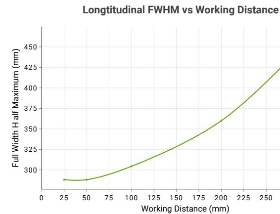
Both Full Width Half Maximum (FWHM) vs Working Distance plots shown above have been measured using a 12-inch white BL138 unit.
