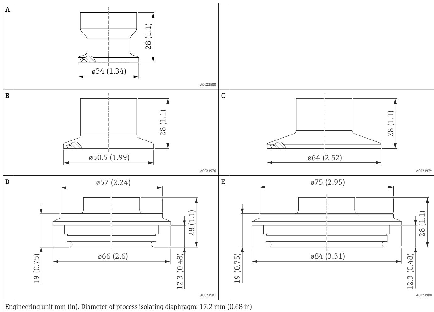
Engineering unit mm (in). Diameter of process isolating diaphragm: 17.2 mm (0.68 in)
