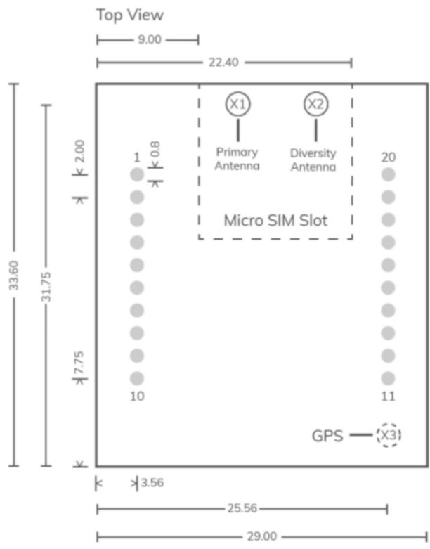
**Note:** U.FL locations are marked with circles. X1 and X2 are located on the top side of the board. X3 is the GPS antenna connector, but is not populated on the non-GPS "-NG" variants of the NL-SW-LTE-SRC7611-4 modem family. J3 is the micro SIM card slot on the bottom side of the board.
