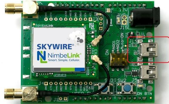
The USB to serial UART IC is an FTDI FT234XD. The FTDI drivers for the FT234XD are available on [FTDI's website](https://www.ftdichip.com/Products/Serial%20Interface%20ICs/FT234XD.htm).
