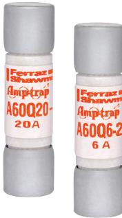
A60Q Amp-Trap® Form 101 high speed fuses feature the only 600V AC / DC rating in the industry of similar size (1-1/2" x 13/32") fuses protecting semiconductors. A60Q also has the lowest I<sup>2</sup>t of all similar fuses and excellent cycling ability. Applications include inverters and small equipment requiring extremely fast response to faults, without the need to carry sustained heavy overloads.
