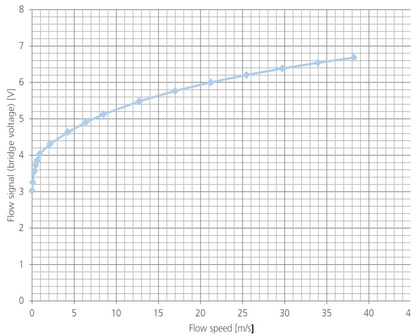
The output signal is adjusted to 3.0 V at zero flow and corresponds to a temperature difference (heater temperature minus ambient) of approximately 30K. With the temperature difference an optimal overhead of the heating element is generated and hence a perfect performance exists. According to King's Law, which is declared in section 1.12, the sensor performance has the highest sensitivity at lower flow speeds.
