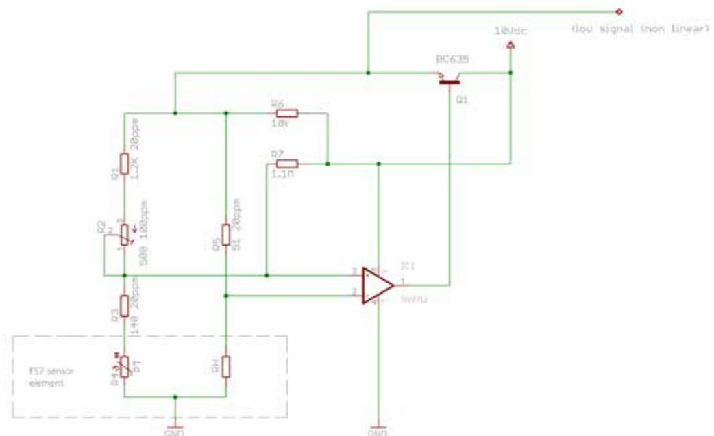
Electronic circuit and curve progression are examples. Each application linked to the accuracy level requires an individual calibration of the system.
