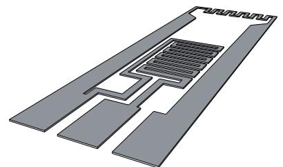
The sensor is individually laser trimmed to the customer specific resistance.
