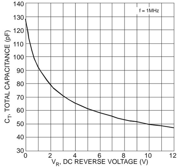
Figure 4 Typical Capacitance
