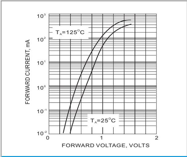
**Fig.3 FORWARD CHARACTERISTICS**
