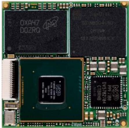
The i.MX 8XLite SoC based LGA Module is designed as per the Open Standard Module™ specification (OSM). It integrates NXP's i.MX 8XLite offerings Dual/Solo Cortex A35 @ 1.2GHz, advanced multicore processing with V2X acceleration supported by Arm® cores.
