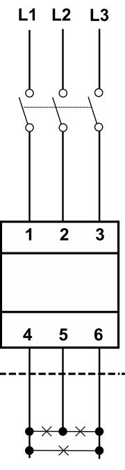
**Fig. 4** Three-phase without neutral (3-wire). MID
