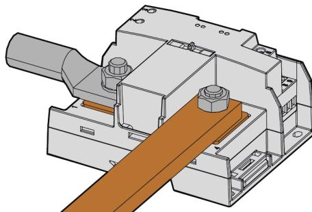
*Fig. 2 Horizontal screw-bar mounting*
