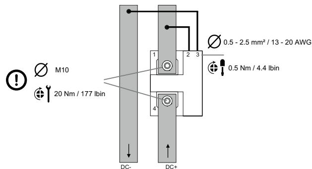
**Fig. 10** Current (option A) and voltage inputs
