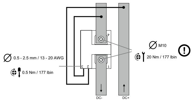
**Fig. 11** Current (option B) and voltage inputs
