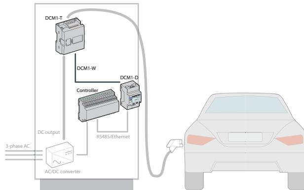
DCM1 connects to the controller via Modbus communication. All relevant information about the charging session is displayed on the screen and recorded in the OCMF file, making DCM1 an ideal solution for installation in EV chargers. The product is compliant with MID, Eichrecht, and A.F.I.R. standards (For more information about charging session see the user manual).
