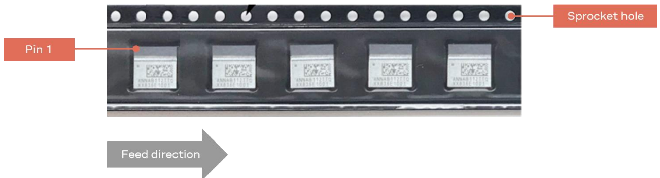
Figure 7: Orientation of ANNA-B112 modules on tape
