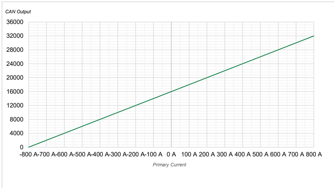
$$\{\text{CAN\_Output}\} = (\{\text{Primary\_Current}\} - \{\text{Offset}\}) / \{\text{Factor}\}$$
