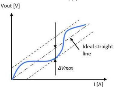
$$\varepsilon_L = \pm \frac{\Delta V_{max}}{V_{FS}} \times 100\%$$
