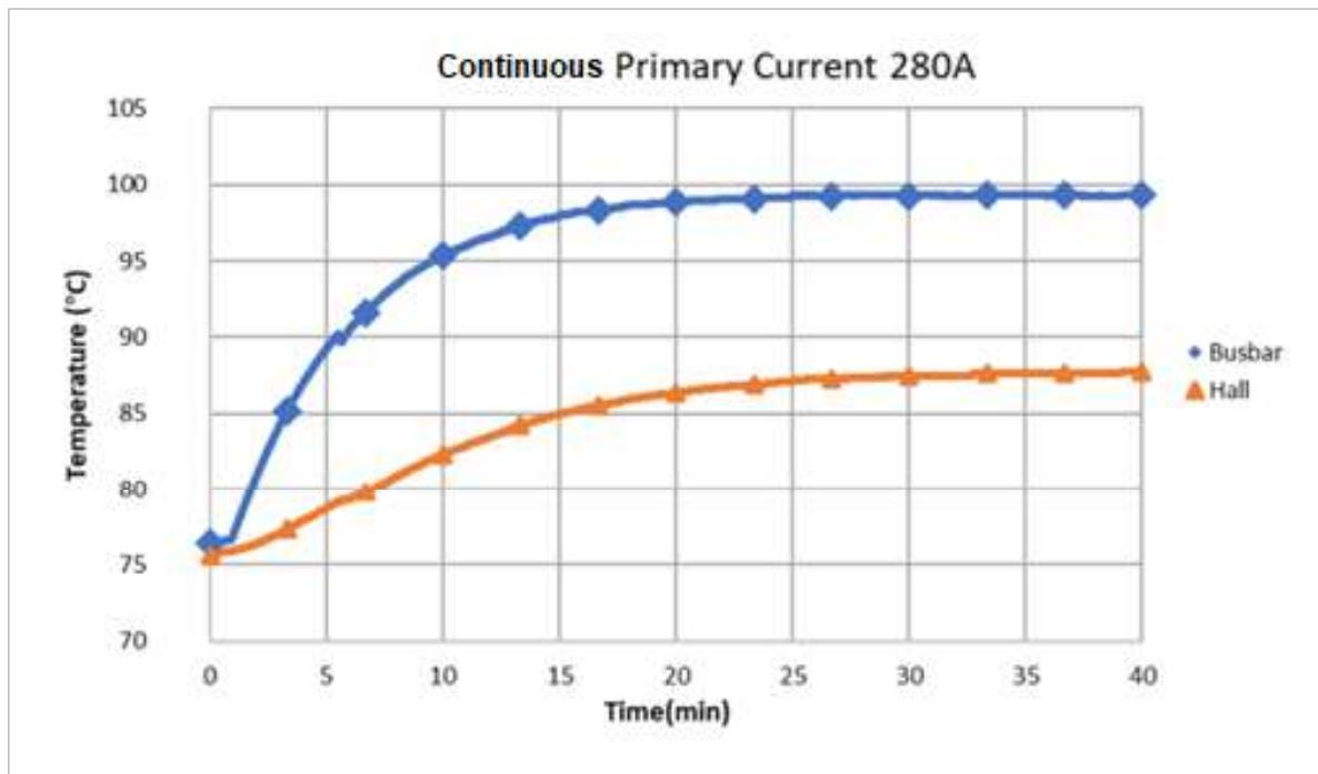
This test is started from 85°C ambient temperature. Heat rise could be verified by other primary current value.
