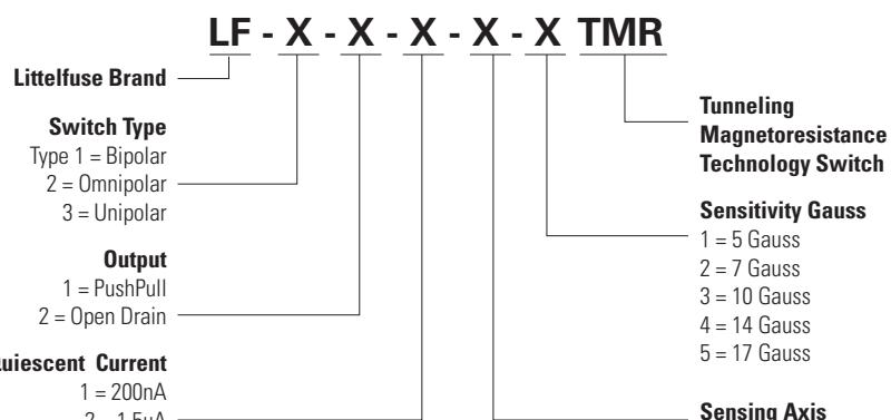
**Example:** LF21115TMR is an Omnipolar, PushPull, 200nA, X axis, 17 Gauss
