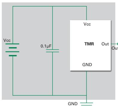
**Note:** It is strongly recommended that an external bypass capacitor be connected in-close-proximity to the device between the supply and ground pins to reduce noise. The recommended value for the external bypass capacitor is 0.1μF.
