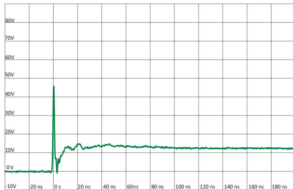
IEC 61000-4-2 +8 kV Contact ESD Clamping Voltage
