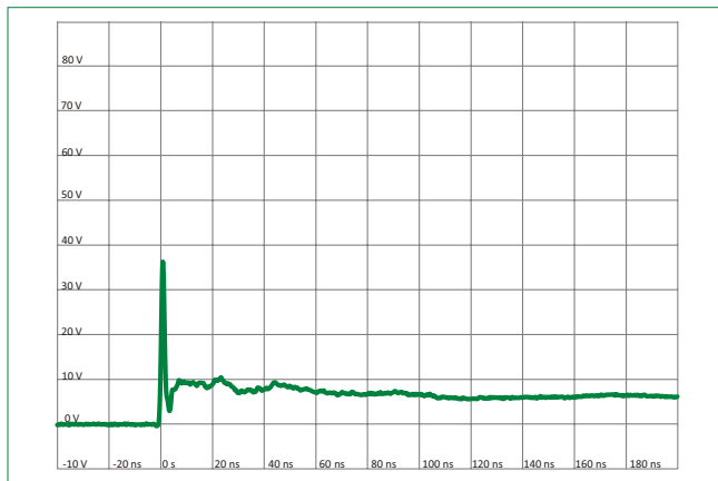
IEC 61000-4-2 +8 kV Contact ESD Clamping Voltage
