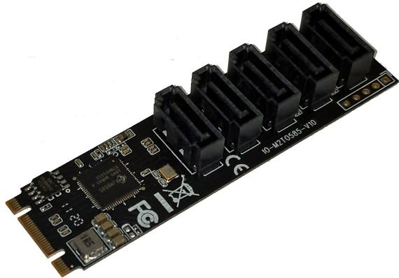
Please note: This is a SATA controller card only – no hardware RAID function is provided. Software solutions such as Linux md or btrfs may be used to provide redundancy.
