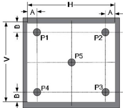
*Measuring method for Contrast ratio, surface luminance,
